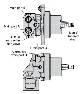
Fan motor (F11-10 left hand rotated shown).
