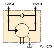
Schematic Fan motor with anti cavitation valve
