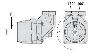
The direction  $(\alpha)$  of the radial load is positive in the direction of rotation as shown.
