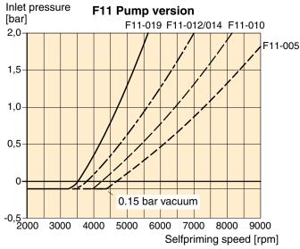
Diagram 2. Min required inlet pressure for Pump.
