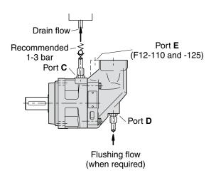
In mounting positions such as 'shaft up' (below) a spring loaded check valve should be installed in the drain line in order to insure a sufficiently high oil level in the case.
